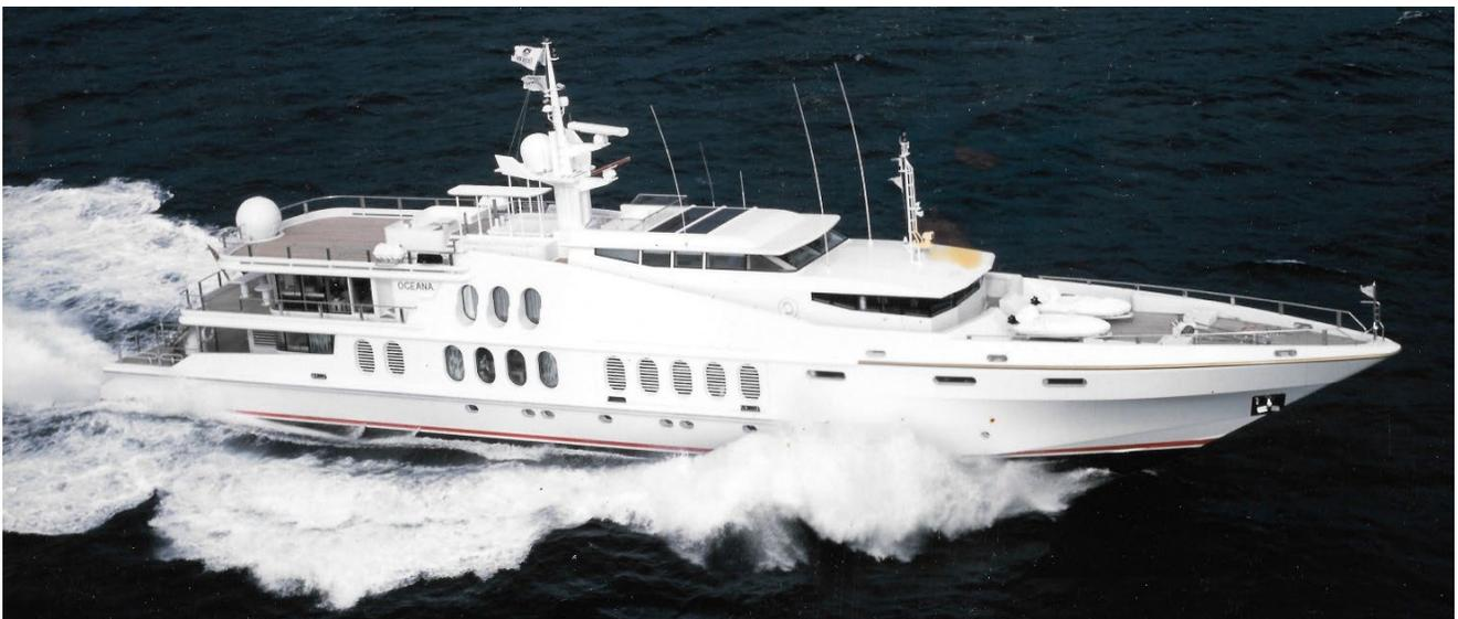
Motor Vessel Bolkiah I / Launched as M/V Oceana C. 180 foot Oceanfast Semi-Displacement Water Jet propelled. 1991
